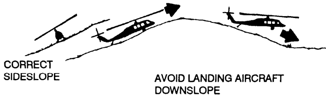
Figure 4-2. Determining ground slope.
